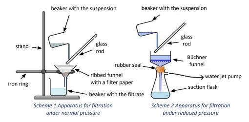
**Equipment:** beakers (150, 250, 400 ml), watch glass, graduated cylinder (100 ml), water jet pump, Büchner funnel, suction flask, ribbed funnel, iron ring, filter paper, scissors, glass rod, spatula, crystallising dish
